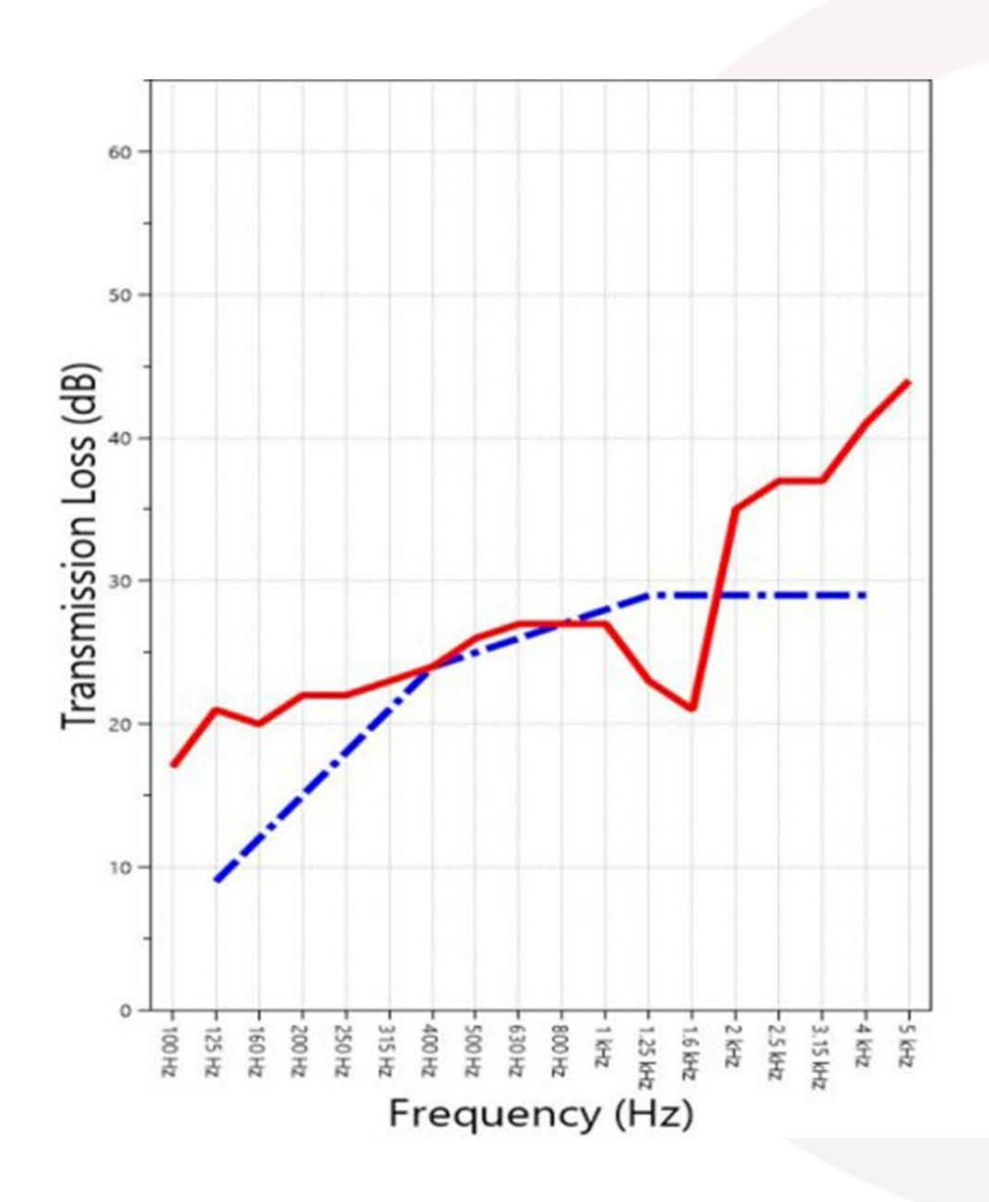
Sound testing was completed at an accredited U.S. Department of Commerce, National Institute of Standards and Technology lab. Across all frequency's tested Barrier Fence sound wall had an average transmission loss of 27 dB. Scoring an STC rating of 22, and an OITC rating of 23.
