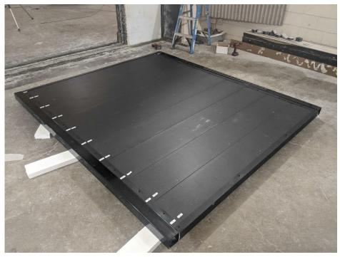
Figure 6 – Test specimen assembled, prior to installation in test aperture
