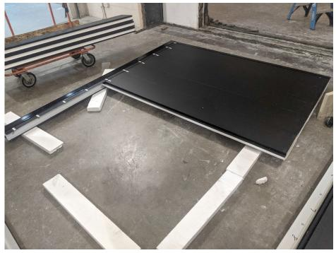
Figure 5 – Test specimen planks fit into framing
